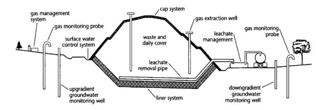
Figure 1.1: Schematic of a Typical Sanitary Landfill (UNEP, 2005)
